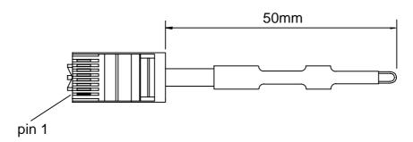
Figure 3-19. CAN Bus Terminator
